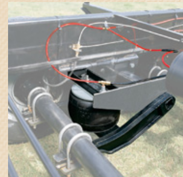
Smooth out the road with this independent Air Ride suspension system, acting in tandem with a torsion axle, that puts each tire on its own active cushion of air — filling and releasing as needed.
