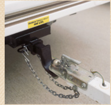
The boat hitch doubles as a receiver hitch for a bicycle rack.
