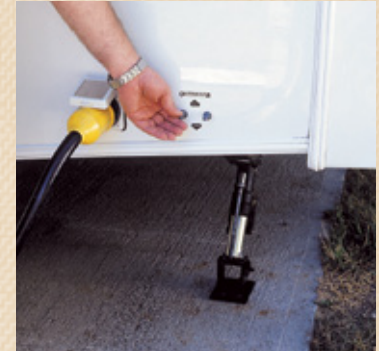
Electric stabilizer jacks make set-up a breeze and saves your back and shoulders.
