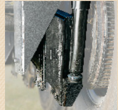
The Mor/ryde (rubber independent suspension) system replaces the standard leaf spring suspension to provide smooth towing and better protects your RV from road shock.
