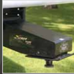
The Glide Ride Pin Box absorbs bumps and jolts through a gravity, self-centering parallel linkage system.
