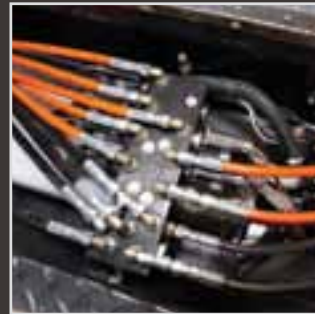
Our uni-body hydraulic valve system for slide rooms and jacks include individual functionality and a manual override.
