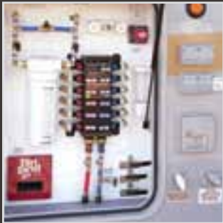
Our multi-function utility center provides easy access to shut off individual faucets, change water filters, replace vacuum bags, disconnect the battery and more.
