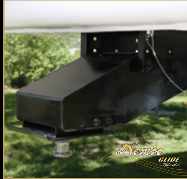
The Glide Ride Pin Box absorbs bumps and jolts through a gravity, self-centering parallel linkage system.
