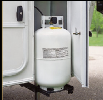
Slideout propane compartments on each side of coach keep tanks secure, and make the controls easy to read and reach.
