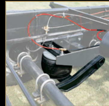
Smooth out the road with this independent Air Ride suspension system, which puts each tire on its own active cushion of air –filling and releasing as needed.
